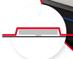
Profiline membrane keypads Height: approx. 1.0 - 1.5 mm*
